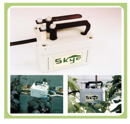
The design of the EvapoSensor was initialised by Horticulture Research International at East Malling, Kent, UK. The 2 simulated leaves are affected by their local environment just like plant leaves, and react to the four weather factors which drives water loss from plants, namely relative humidity, air temperature, wind speed and solar radiation.
