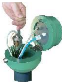
simple battery change without tools at the system "LogCom"
