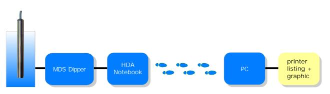
Of course, the data logger MDS Dipper-T3 can be connected directly to a PC (i.e. Notebook) or to a data transmission modem, due to serial interface.
