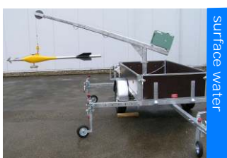
SEWII with mobile jib and current meter
