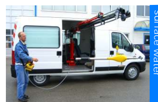
vehicle with crane and current meter
