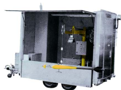
trailer with mechanical or electrical SEW - II for measurements from bridges
