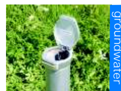
Open Top Piece with installed Data Logger
