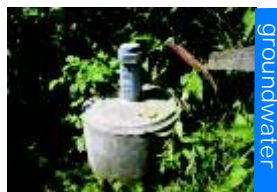
Top Piece with GSM antenna
